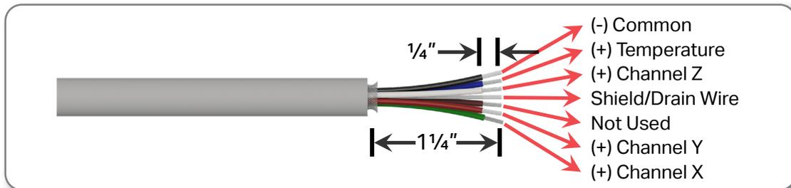
4. Locate the appropriate plug, identified by channel number, remove the plug and install the wires using a small flathead screwdriver. Push plug back into location.
