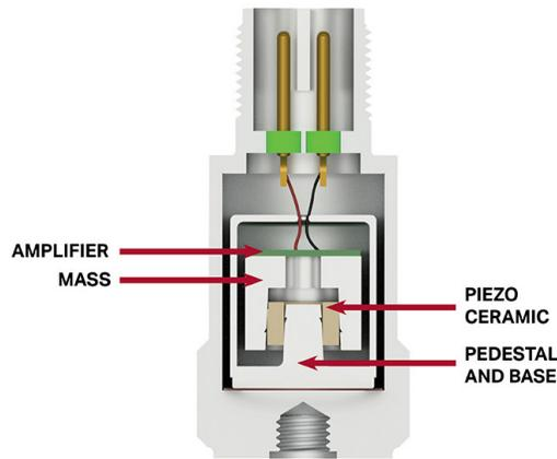
In a shear mode design, no stud holds the internal components together. Most designs use a form of epoxy cured under heat to maintain structure. The base and the mass have no contact, so there is no metal-to-metal contact within the sensing element, which significantly reduces the impacts of thermal transients.
