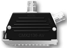
25 Pin Adapter with Dual BNC "E" Jacks, Channel "1" Acceleration Input, Channel "2" Voltage Input, 221 °F (105 °C) Maximum Temperature, Compatible with CSI 2130 Data Collector
