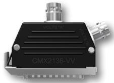
25 Pin Adapter with Dual BNC Jacks, Channel "1" Voltage Input, Channel "2" Voltage Input, 221 °F (105 °C) Maximum Temperature, Compatible with CSI 2130 Data Collector
