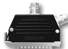
25 Pin Adapter to Dual BNC "E" Jacks, Channel "1" Acceleration Input, Channel "2" Voltage Input, 221 °F (105 °C) Maximum Temperature, Compatible with CSI 2120/2130 Data Collector
