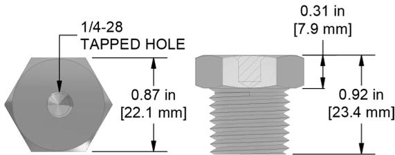
1/2-14 NPT Plug with 1/4-28 Blind Tapped Hole, 316L Stainless Steel, 0.61 in. (15.5 mm) Length, 0.87 in. (22.1 mm) Diameter
