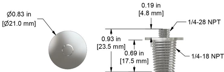
1/4-18 NPT Plug to 1/4-28 Adapter Stud, 316L Stainless Steel, 0.93 in. (23.5 mm) Length, 0.83 in. (21 mm) Diameter
