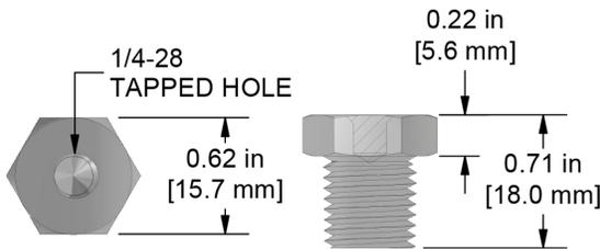
1/4-18 NPT Plug with 1/4-28 Blind Tapped Hole, 316L Stainless Steel, 0.49 in. (12.4 mm) Length, 0.62 in. (15.7 mm) Diameter
