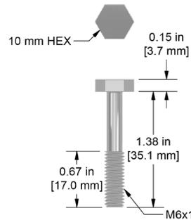
M6x1 Captive Bolt for 500 mV/g, 1000 mV/g Side Exit Sensors, 18-8 Stainless Steel, 1.38 in. (35 mm) Length
