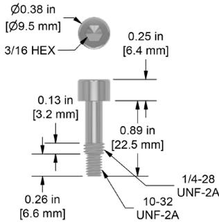
10-32 Adapter Bolt with Socket Head Cap for CTC AC119, AC115, AC230 and AC360 Sensors, 18-8 Stainless Steel, 0.89 in. (22 mm) Length
