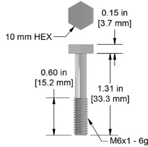
M6x1 Captive Bolt for Standard Side Exit Sensors, 18-8 Stainless Steel, 1.31 in. (33 mm) Length
