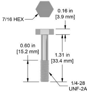
1/4-28 Captive Bolt for Standard Size Side Exit Sensors, 18-8 Stainless Steel, 1.31 in. (33 mm) Length
