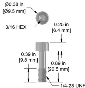
1/4-28 Captive Bolt with Socket Head Cap for CTC AC119, AC115, AC230, and AC360 Sensors, 18-8 Stainless Steel, 0.89 in. (22 mm) Length
