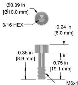
M6x1 Captive Bolt with Socket Head Cap for Miniature Industrial Side Exit Sensors, 18-8 Stainless Steel, 0.75 in. (19 mm) Length
