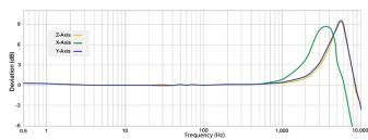
25.6 kHz sampling frequency is required to utilize full bandwidth shown
