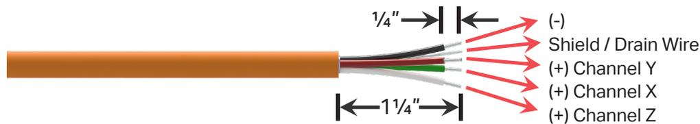
**Figure 9. Stripped Wire**
