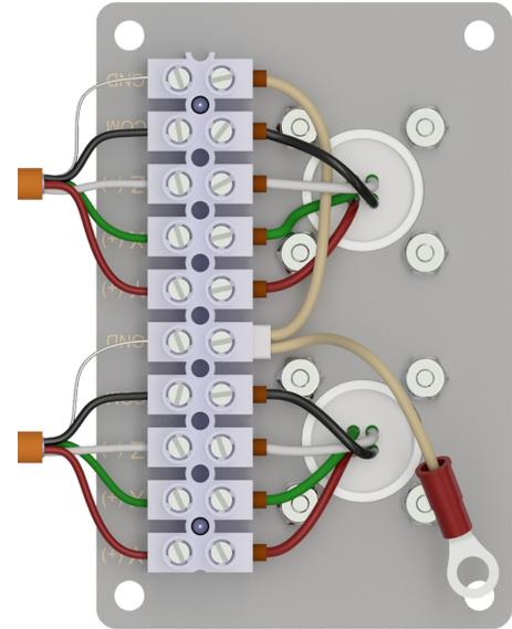
**Figure 10. Field Wiring for Four-Conductor Triaxial Sensor Inputs**
