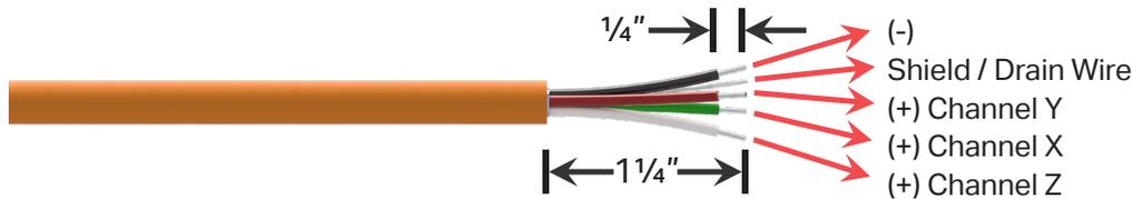
**Figure 9. Stripped Wire**
